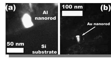
Al, Au and bilayer nanocolumns deposited through porous alumina templates
