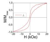
Hard Magnetic nanoparticles on SiO<sub>2</sub> for hard disks with capacities of 11,43Tbit/inch<sup>2</sup>
