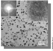
ZnO nanodots, uniformly grown on Si with controlled sizes 3-50 nm Superlattices and Microstructures, 2006, 39 (1), 115-123
