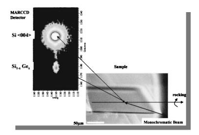
Structural characterisation of selectively grown heteroepitaxial SiGe layers with lateral dimensions in the 1 micron scale
