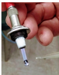
Fig.1. Photograph of the immersible photonic chips, which can be used either as immersible probes or by simple drop casting of the liquid sample
