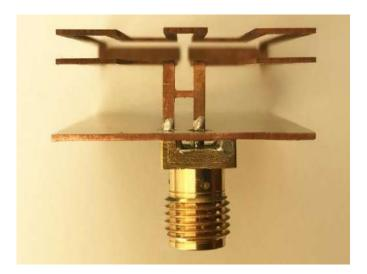
Figure 1. Photograph of the fabricated design D1 showing details of the SMA connector and feed.
