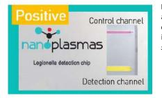
**Fig. 7.** Lab-on-a-Chip for accurate and fast results in the detection of *L. pneumophila*, addressed to the water analysis market. It achieves results in 70 min from sample collection to decision, instead of 10 days using standard microbiological methods. It is a molecular diagnostic technique, a nucleic acid amplification test (NAAT) with *insitu* capture, lysis, specific DNA amplification and naked eye detection.
